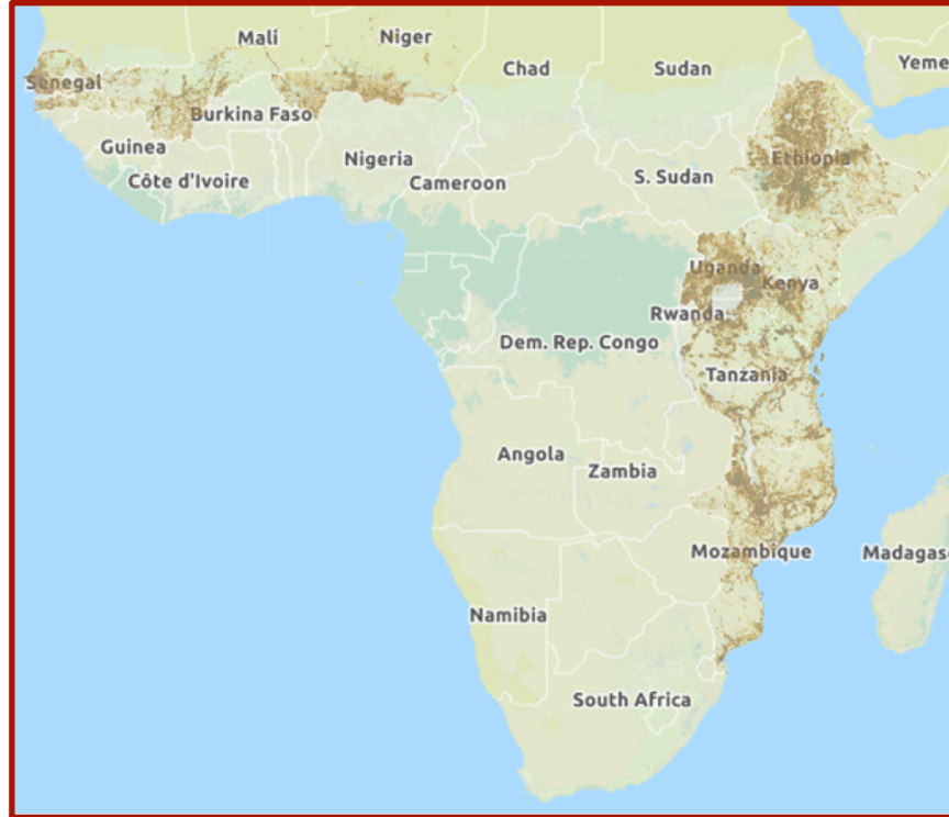
Figure 1 - Distribution of the number of buildings from the African nations currently featured in GED4ALL, following an evenly spaced grid with a 15x15 arcsec resolution.
